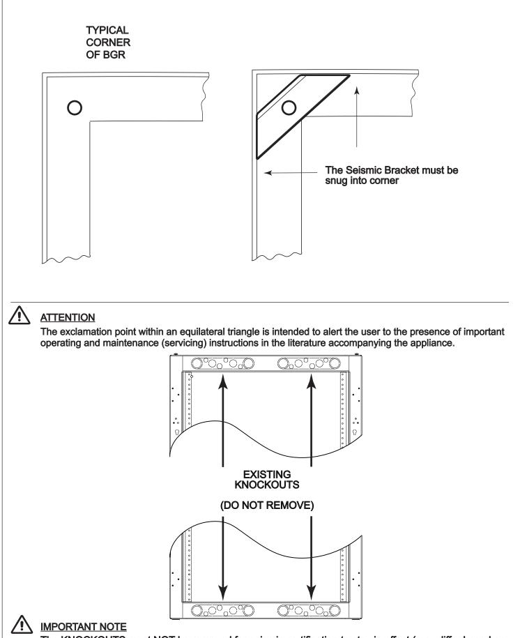
The KNOCKOUTS must NOT be removed for seismic certification to stay in effect (may differ based on enclosure). Enclosure must be plumb and level in 2 directions.
