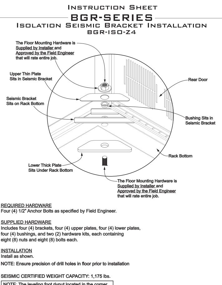
NOTE: The leveling foot rivnut located in the corner does not need to be removed. Tighten the floor anchor completely. Deflection will occur around the rivnut. This is required, it pre-loads the corner in compression.
